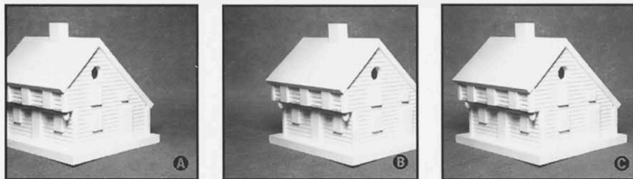
If the subject looks like A on the ground glass, or like B , use the front or back lateral shift, and the subject will look like C , properly composed. Note: Moving the back shift does not change the camera's point of view in relation to the subject. Shifting the front, or lens, does alter the camera's viewpoint, affecting the relationship between near and far subjects.
