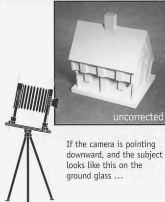
1. Tilt the camera back parallel to face of the subject to correct perspective. 2. Tilt camera front parallel to back to correct sharpness. Refocus if necessary and the subject will look like this.
